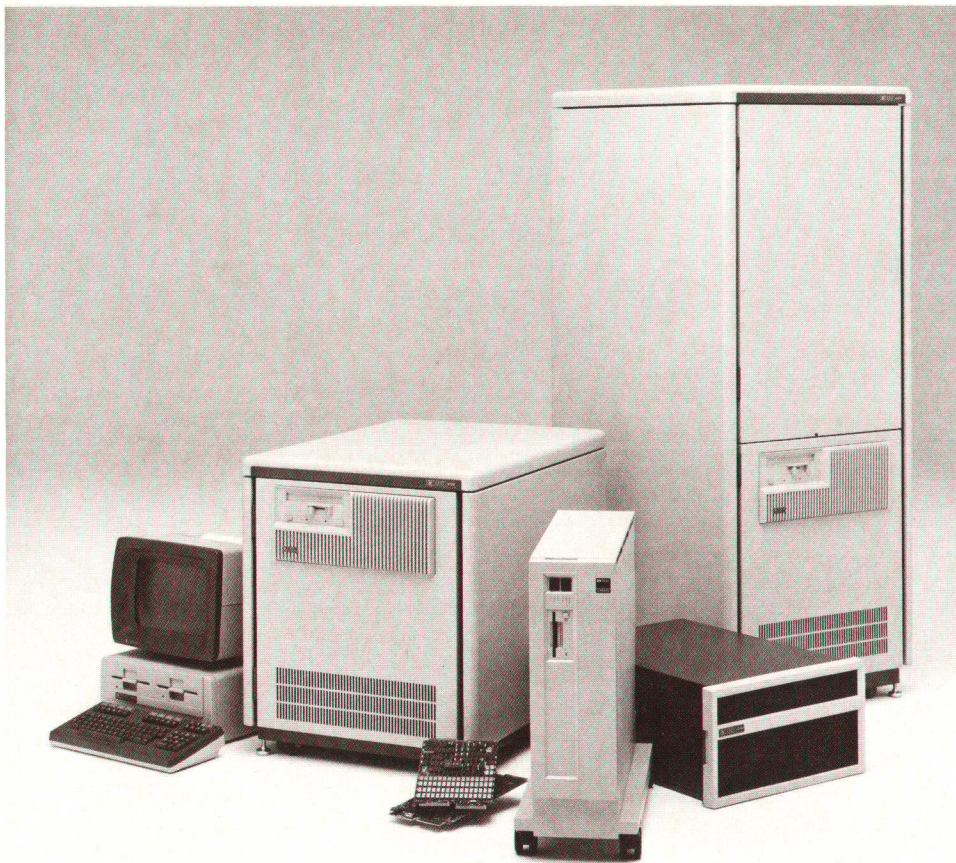
Fig. 1. HP 1000 A-Series Computers come in various configurations and have performance ratings ranging from 1 to 3 million instructions per second.
